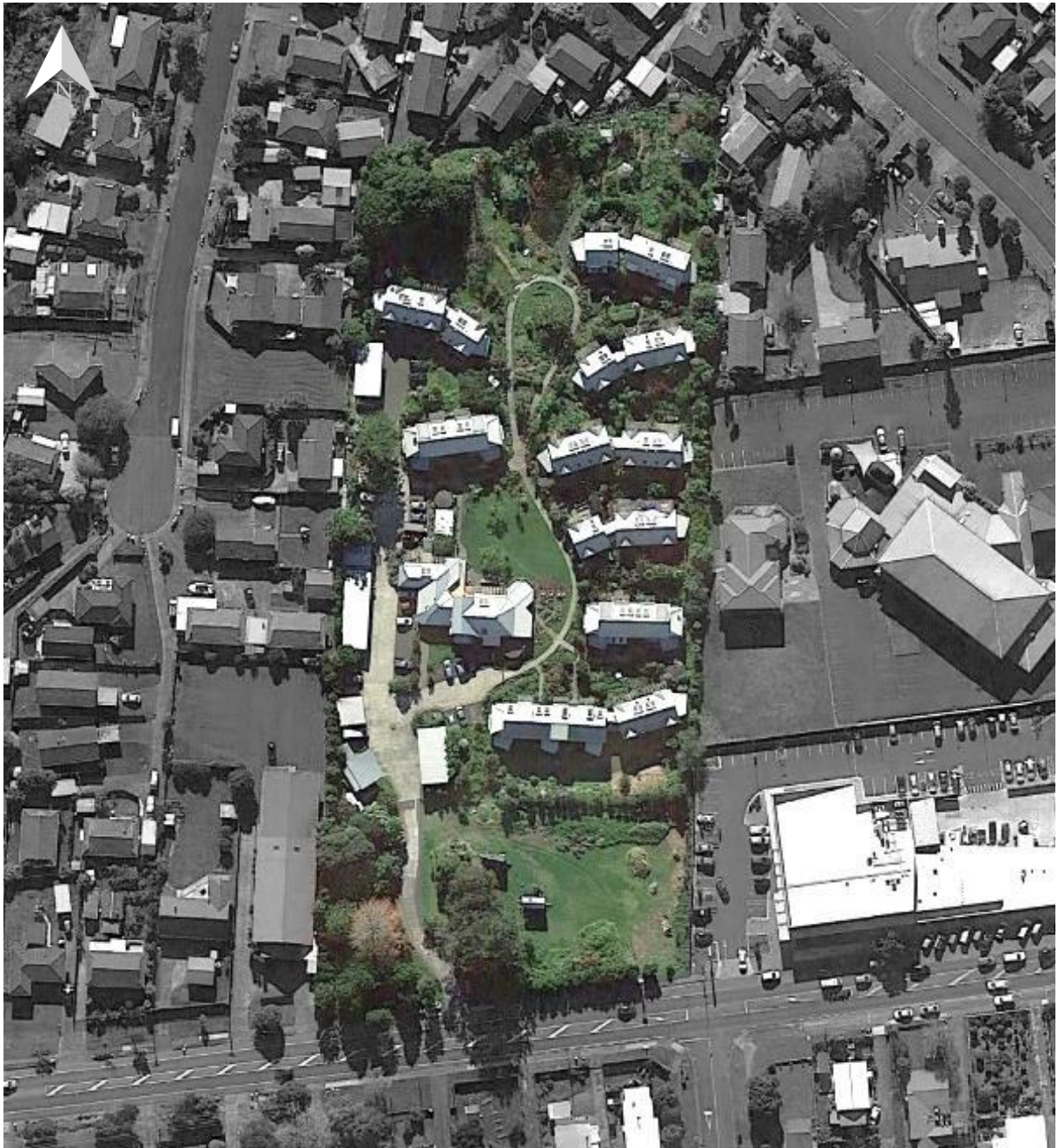
Figure 10: Earthsong Eco-Neighbourhood aerial photo (development shown in colour). The aerial photo illustrates how clusters of homes are elongated east-west to provide north-facing living areas in each unit. Car-parking is kept to the Western edge of the site, keeping the network of footpaths available for pedestrians.
